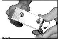
**7.2.4** Using three (3) no. 8 x 1/2" screws provided with hood, secure the adapter to the back of the cabinet blower. Remove tape from damper flap. Seal the adapter and the metal shutoff plate to the cabinet blower using duct tape.
